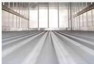
T-type air-ducting bottom rail patterned aluminum sheet
