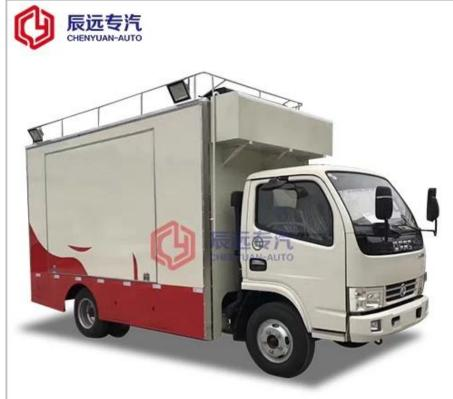
Production Name: Mobile food truck Production brand: Dongfeng brand Drive direction: Left hand drive Production model: HCQ5040XCCDFA Overall size(mm): 5995 \* 2090 \* 3300 Cabinet size(mm): 4200x1800x1850 Bear Weight: 2T ~ 3.5T Gearbox: 5 forward and 1 reverse Engine model: CY4102-C3F Spray Color: Any Color
